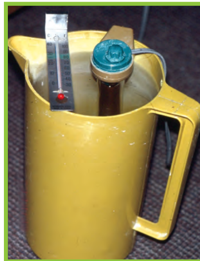
Figure 2. Fish tank heater will maintain constant water temperature in the juice canister.
